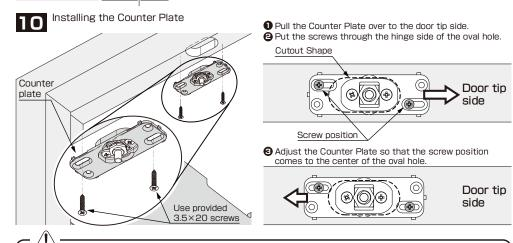
Do not open or close the door before adjusting the installed counter plate. Operating the door without counter plate adjustment may result in malfunction, causing damage to the damper, door or frame.
