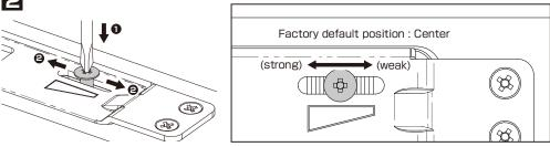
Firmly tighten the Damper Force Adjustment Screw after adjustment completed.
